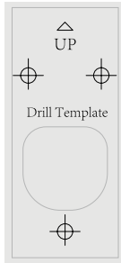
Drill Template for Intercom Panel x1
