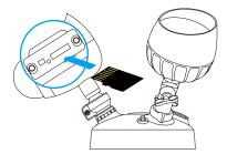
1) After installing the micro SD card, you should initialize the card in the EZVIZ app before using it. For detailed operation, refer to page 5: Initialize Micro SD Card.
